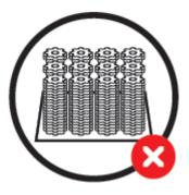
To protect bulk parts or large volume packages, place VCI diffusers in addition (VCI paper, VCI Noxy diffusers, VCI foams, etc.)
